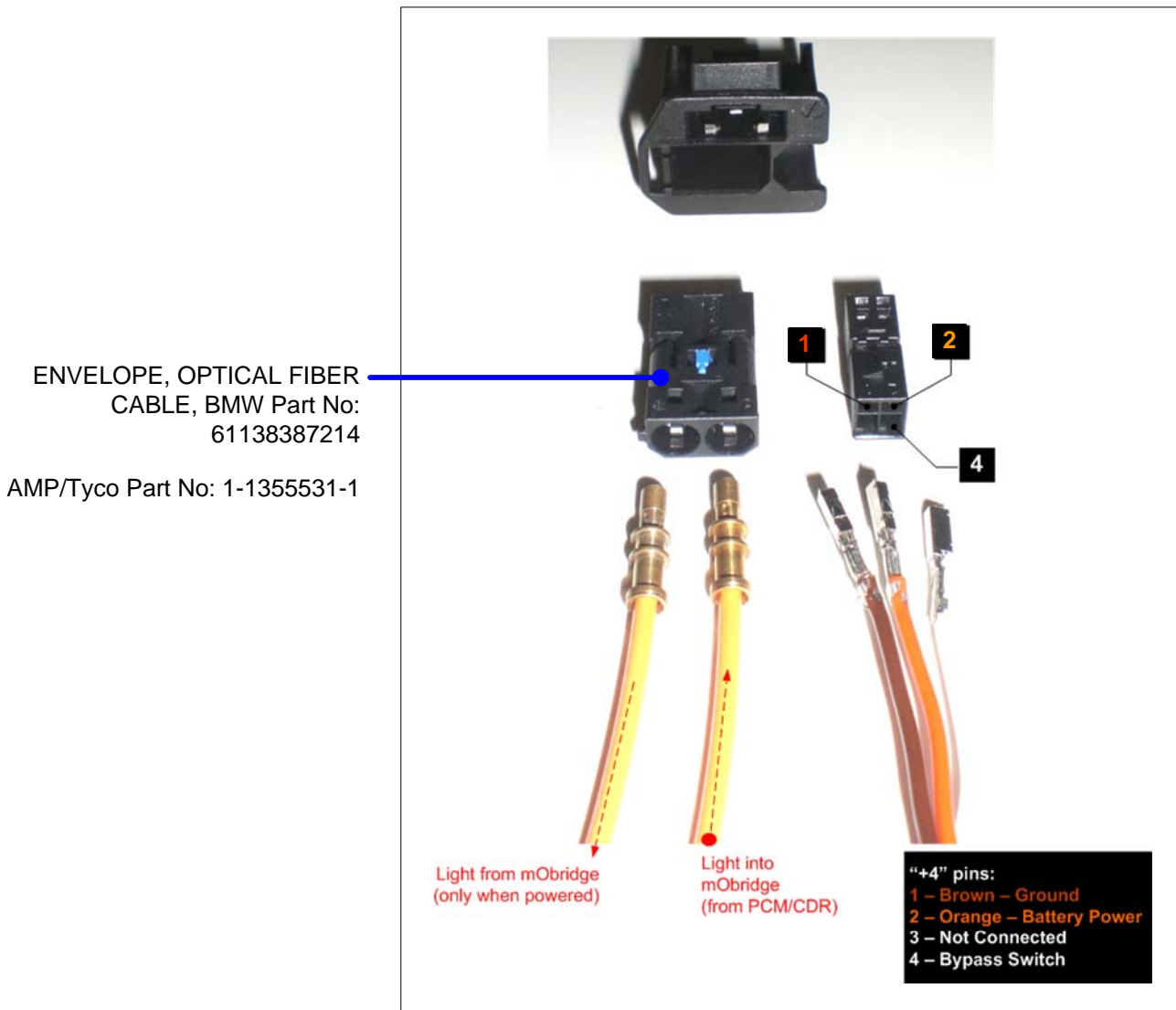
View looking from the back of the 2+4 (Optical + Electrical) connector that plugs into mObridge.
