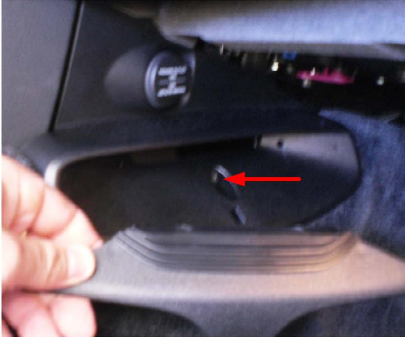
In the passenger footwell against the center console some vehicles have the Bose subwoofer assembly. This assembly blocks access to the center console to an area where installer may wish to route wiring or fiber-optic.
