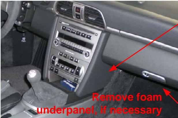
mObridge unit is installed behind the climate control unit and below the CDR24, accessible via this panel.
