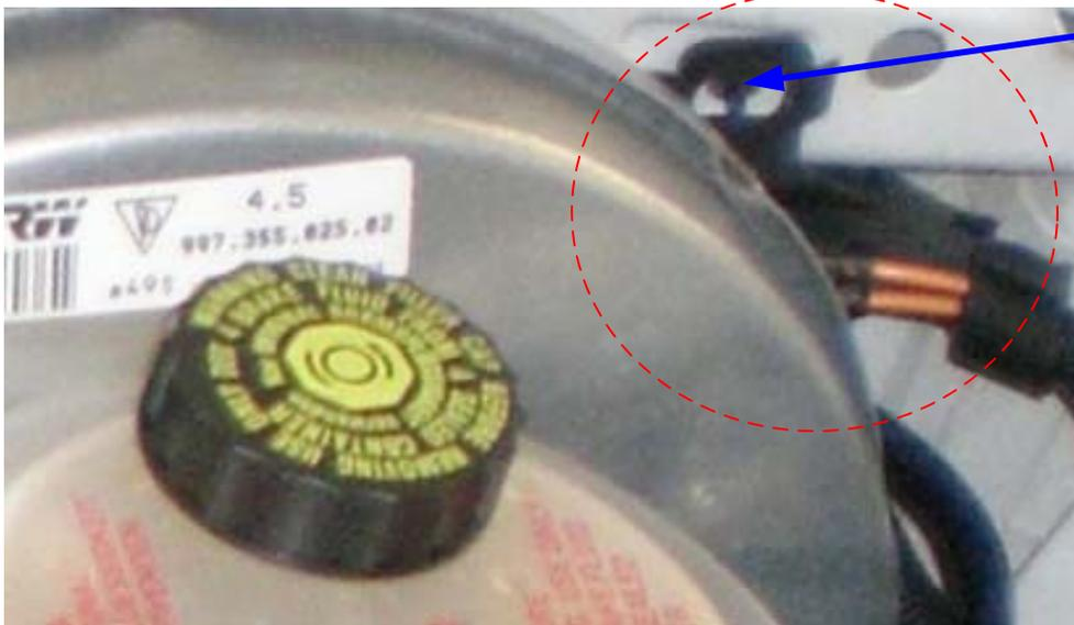
Plastic bracket holding connector (and bypass loop when applicable) can be unsnapped here with needle-nose pliers to get sufficient access,
