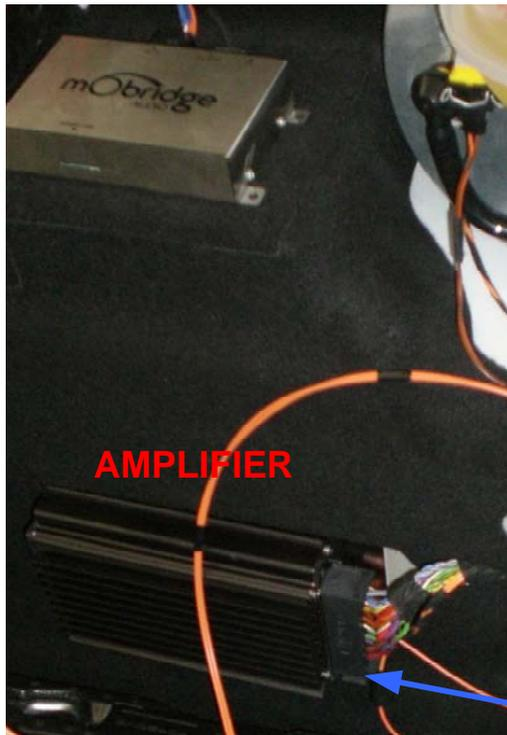
MOST connector is down here (obscured, difficult to see when standing looking at amplifier). It is a 2+0 style with the latch on the side, easy to feel around and remove.
